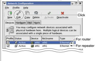
③ Select [Statically set IP address], then enter the specified IP address, subnet mask and default gateway (router side; eth0 setting only), as below. Click [OK], then close "Ethernet Device" screen.
